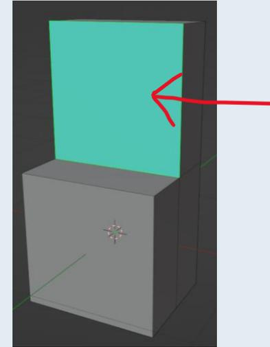
11. Scale the extruded face on all axes to reduce its dimensions
